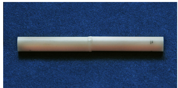
Fig. 12. Joined Al 2 O 3 ceramic.
